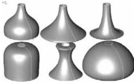
Various combinations of Draft Angles and Draft Magnitudes Skinning Two Circles
