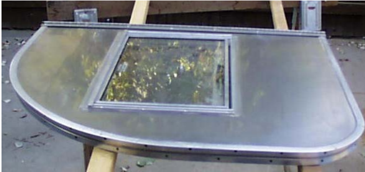
Completed door with trim and hinge attached.
