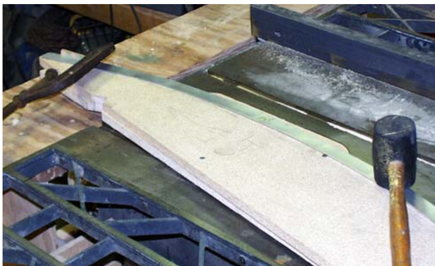
Beating the softened 1" angle around the particleboard form.
