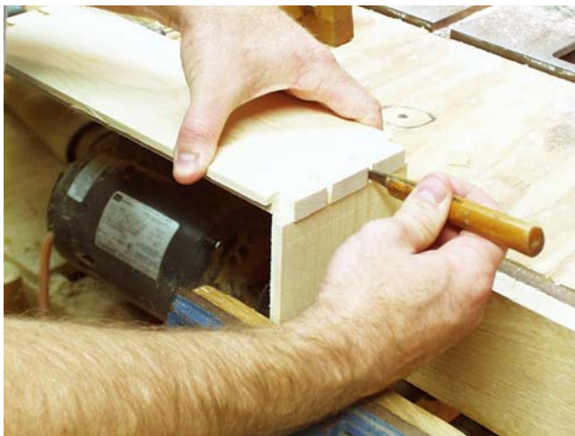
5.) Scribe the tails onto the front or back board to lay out the pins. Using a square, draw vertical lines from the marks you just scribed down to the scribed line.
