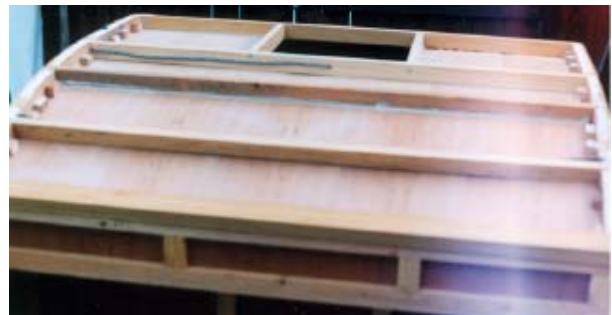
Cross-sighting spars: visually line up the top of one with the bottom of the next one; they should be even.
