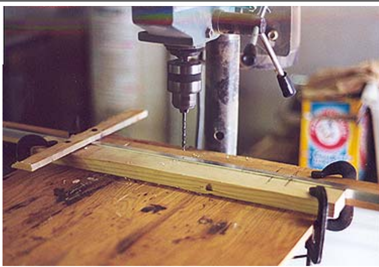
Jig for drilling holes in the trim, basically just two boards that support the trim while drilling. Lines at right are index lines to space the holes. Cross board at left holds the trim down while lifting the drill out.
