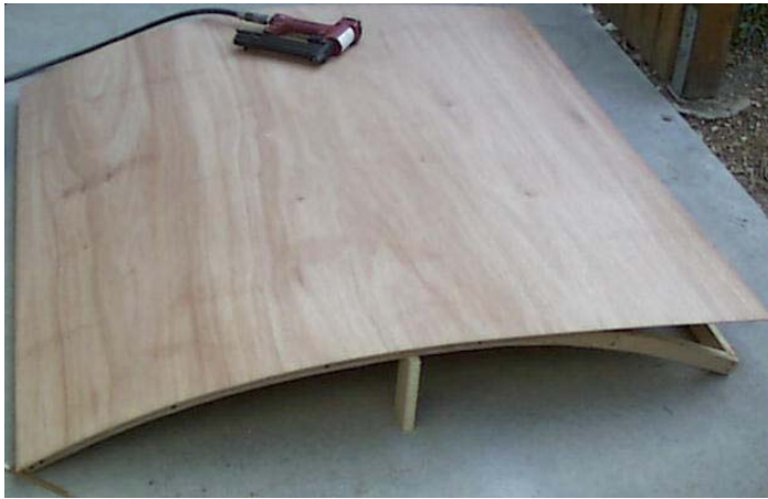
Attach 1/8" skin with glue and brads, starting at the top and working your way down. Notice the support stick holding up the middle.
