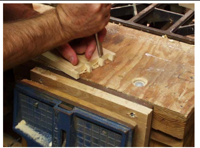
8.) With a sharp chisel, clean up the cuts, paring down to the scribed line.
