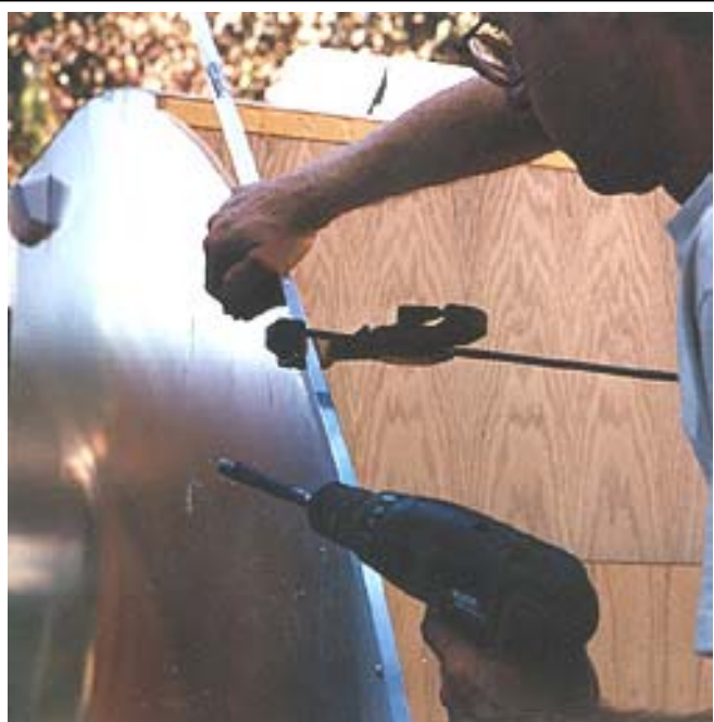
Applying the corner trim. This goes a lot easier if you soften the angle trim by annealing first. Do not caulk the hatch trim yet, as you will remove it later for final shaping of the hatch/body gap.
