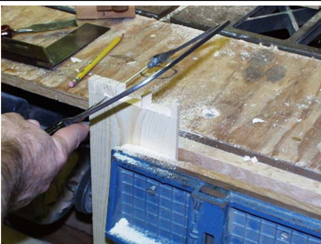
7.) Saw out the waste portions with a coping saw, staying above the scribed line.
