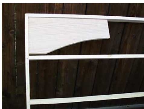
Temporary scrap screwed to the frame corner to ensure squareness.
