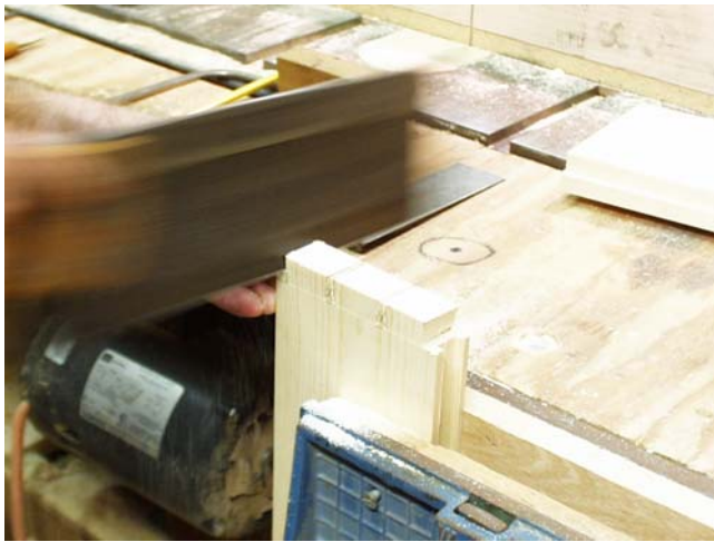
3.) Saw down to the scribed line, being careful to saw on the "waste" side of the lines. Also saw the shoulder cuts on each side.
