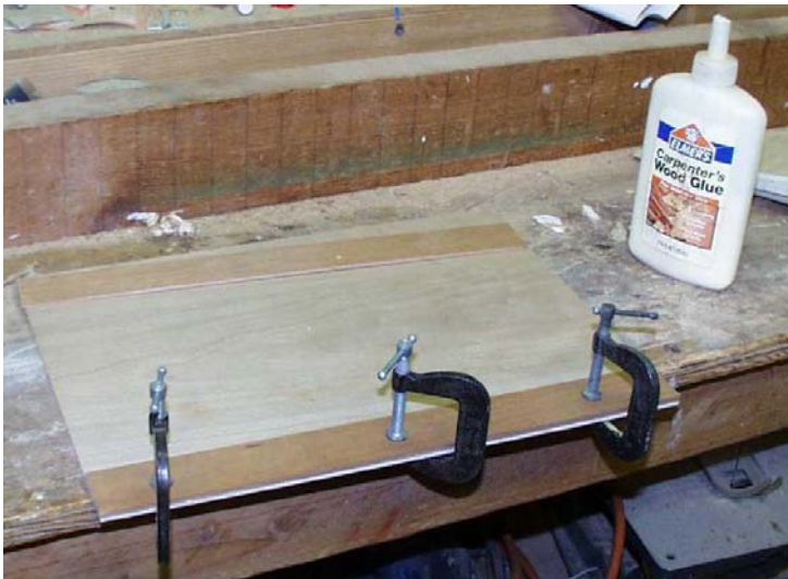
The sliding doors are glued up from 1/8" plywood faced with pieces of 1/8" solid wood to make a total thickness of 1/4". While gluing, clamp the piece against something flat to keep everything straight. See details p. 95
