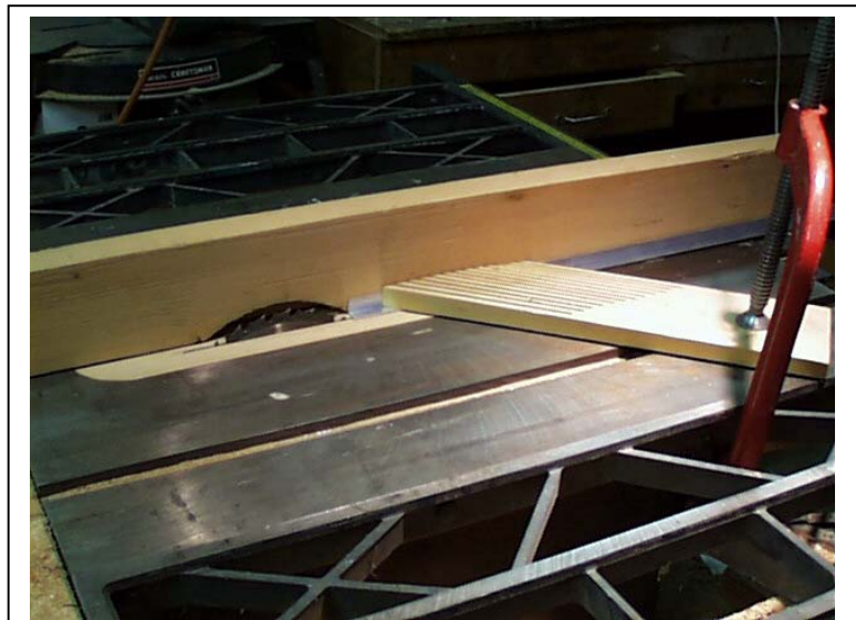
Sawing aluminum trim. Do not attempt this without the featherboard and zero-clearance blade insert. Some thick washers suspend the featherboard just above the saw tabletop, and allow the trim to slide under.
