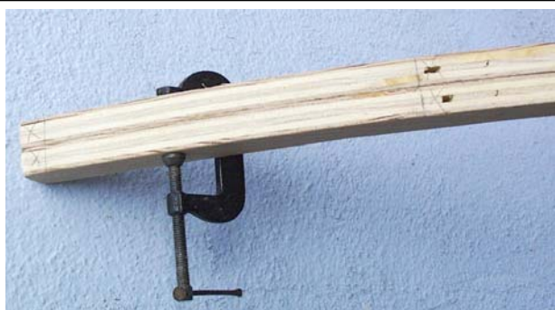
Gussets clamped together for sanding. Layout marks showing where spars attach.
