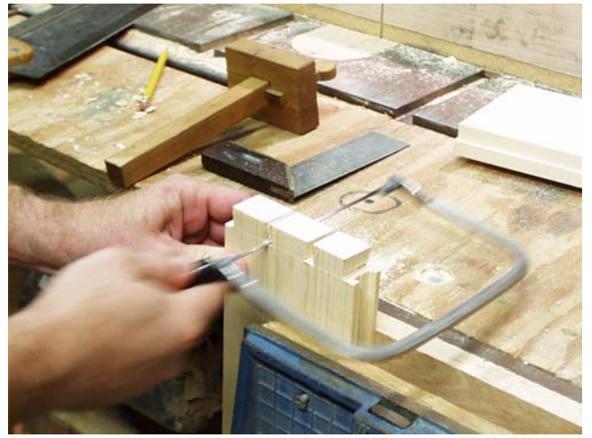
4.) Use a coping saw to remove the wedges between the tails, staying above the scribed line.
