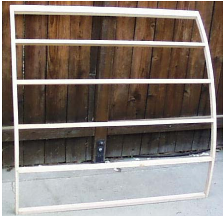
Spars screwed to side gussets. Note the double spar at the top where the hinge attaches. Test the hatch for fit.
