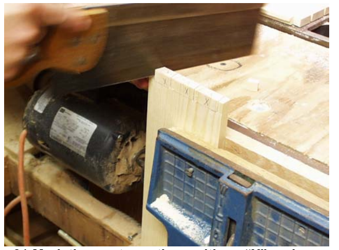
6.) Mark the waste portions with an "X" and saw down to the scribed line, sawing on the "waste" portion of the line.
