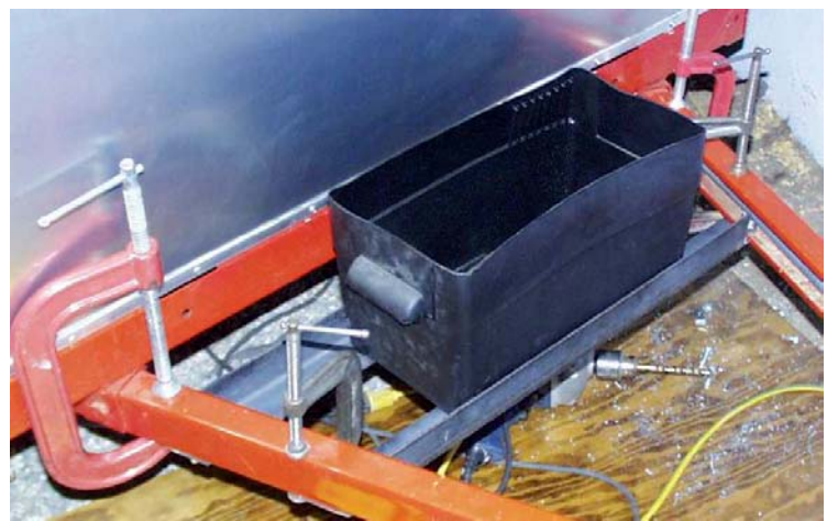
Angle iron clamped in place to check the fit before drilling and bolting in place from below.
