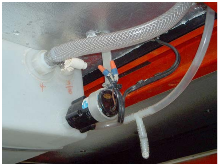
Pump hookup. The pump threads directly into the water tank and is suspended by an aluminum strap. The valve over the 3/8" on the tank is used as a vent, and the "T" fitting is used to drain the tank if needed (or if the battery goes dead!) The large hose is the 3/4" inlet hose.
