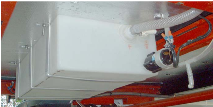
Water tank mounting.
