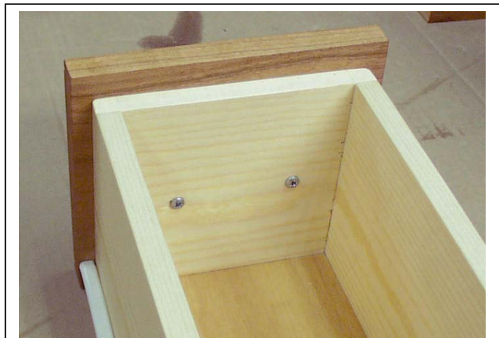
The drawers have a separate drawer front that is attached with screws from the inside.
