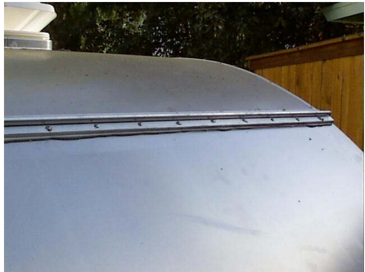
Hatch attached with caulk and 1" stainless screws.
