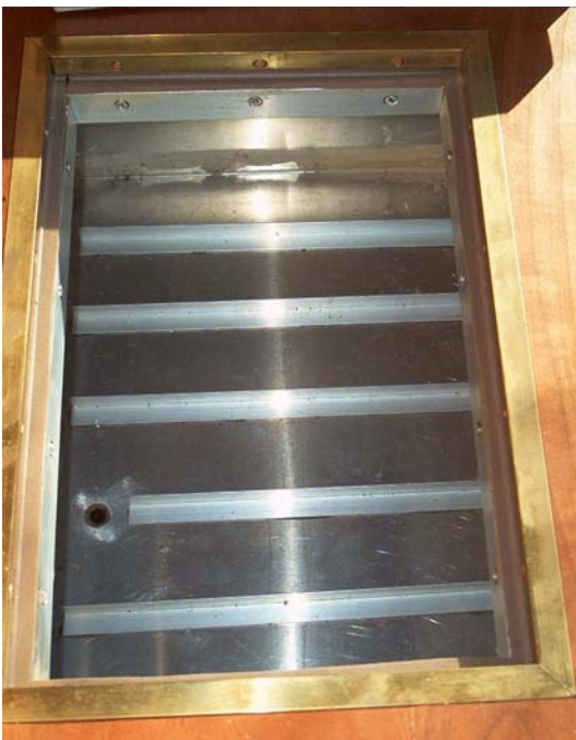
\frac{1}{2} " angle shelf stiffeners epoxied in place.
