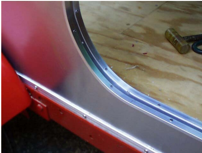
1/2" angle with one leg ripped down to 1/4".
