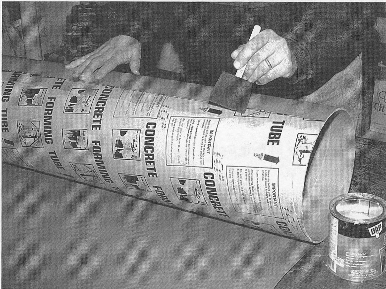
Fig. 13.5 Kydex plastic makes an excellent finish for the tube: it is both tough and waterproof. Recruit a helper. Coat both surfaces with contact cement and allow the cement to dry, then slowly roll the Kydex onto the tube.
