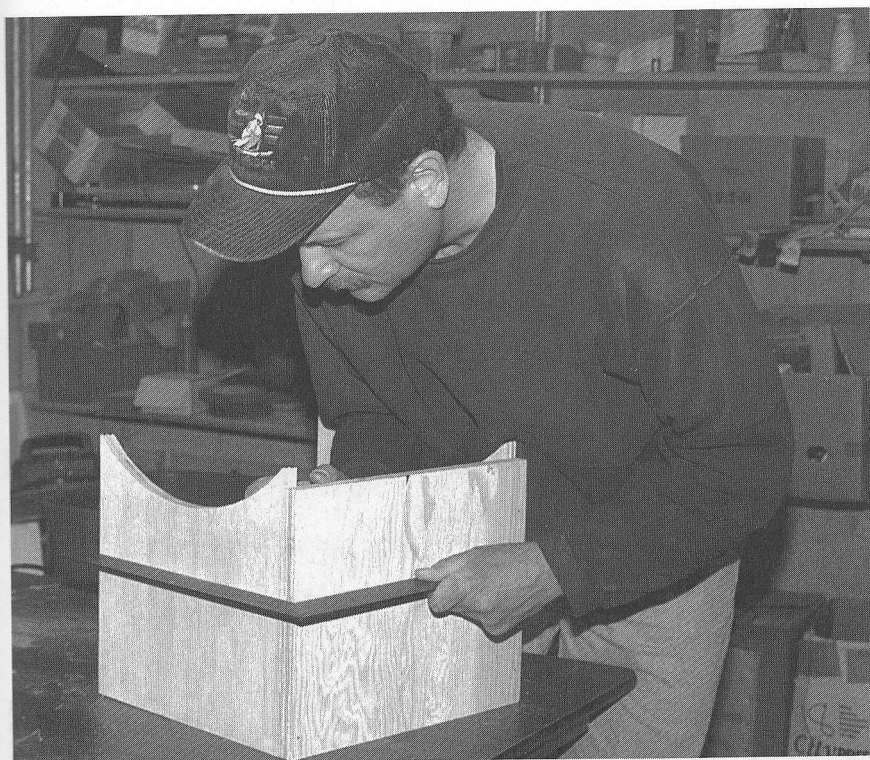
Fig. 13.8 Use a carpenter's framing square to check that the rocker box is precisely square before you put it aside for the glue to set. If the rocker is out of square, the tube cradle may bind against the rocker.
