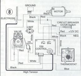
NOTE: The ON/OFF switch, located in line with the gas valve, is not used when a combination circuit breaker and ON/OFF switch is used.
