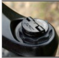
The Deuce fork has a flip up alloy adjustment for setting your preload.
