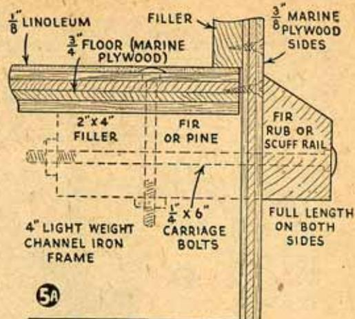
CROSS SECTION SHOWING HOW SIDES ARE FASTENED AT FLOOR LINE.
