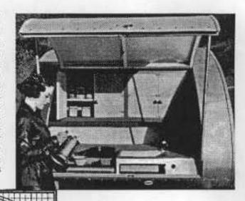
the frame true until entirely assembled. The finished job, with the frames joined by the crossbeams, will appear as in Fig. 6. Casein glue and brass screws are used throughout.
