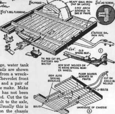
on the care with which you assemble this part of the structure. The housed joints joining the 2 by 4-in, members should be a snug fit. If the joints are an imperfect fit, the vibration and strain to which the parts are subjected will cause them to loosen to such an extent that the lag screws will not hold effectively. Turn the chassis over and set up on sawhorses to keep it steady while going ahead with the construction.
