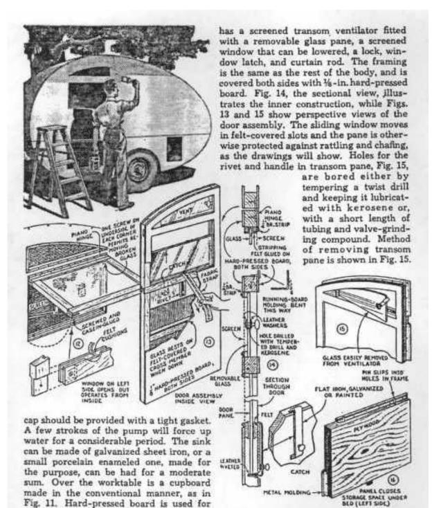
These panes are cut from plate glass with an ordinary glass cutter, and the edges smoothed with an oilstone. The window on the left side is swung out by a bracket on the inside, working through the screen. The transom vent above this is the same as in the door, and the frame assembled as shown, Fig. 12. Also on the left side are two removable panels, one to give access
