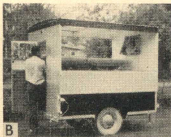
(A) Front erected and roof started up. (B) Roof and ends in place, side wall going up. (C) Raising the last side wall. (Cont'd next page.)
