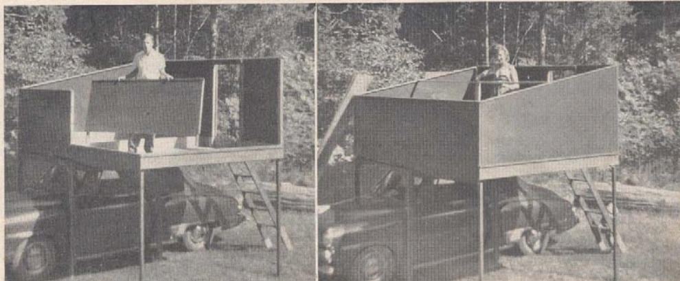
Bolted-together walls hold roof support . . .
