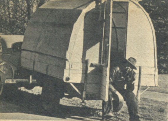
Completed trailer weighs but 450 lbs., so it is easy to handle. Since the road clearance is 18 in., you can take it anywhere your car will go.
